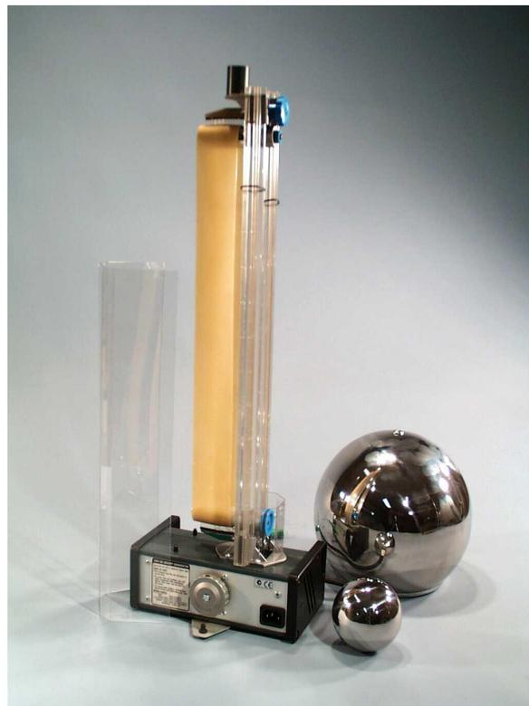
EM4137-001 Van De Graaff generator, 200kV, 200mm diameter aluminium dome
